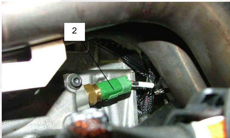
Fit the engine oil temperature sensor (ref. 3) onto the oil pan and connect it to the engine bundle.
