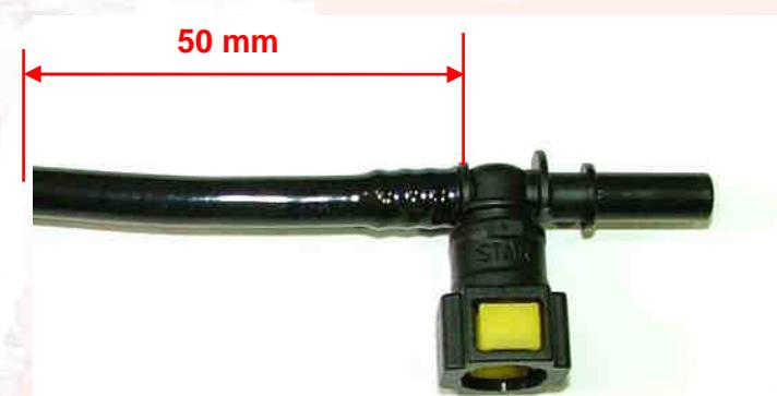
Screw the “fir-tree” connector (chapter A23 “Injection”, page 2) onto the sensor (ref. 4-5), having first coated the threads with *Loctite 577 Thread Sealing*.
